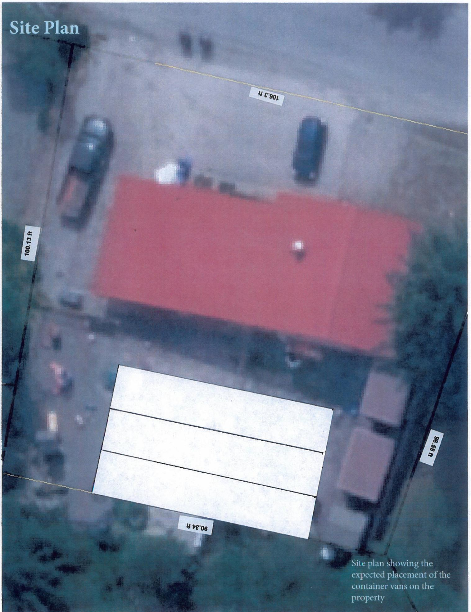
Site plan showing the expected placement of the container vans on the property
